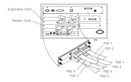
Your analysis probe or processor solution manual does not include information about the pod connections nor about the names of the configuration files for Agilent 16715/16/17/18/19A logic analyzer modules.
